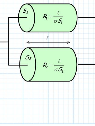
We can view this as a single resistor with a total cross sectional area of  $S_1 + S_2$ . Thus, its total resistance is:
