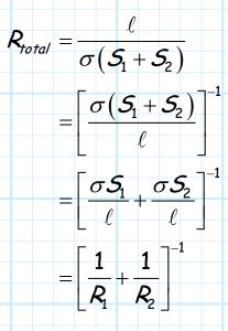
Again, this should be no surprise, as these two resistors are connected in **parallel**.
